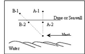
*Figure 2-18. Site A stakes are directly landward of the nest in dune vegetation or at the base of a seawall. Site B stakes are in a similar position as Site A but located at an angle from the nest. Stakes A-1 and B-1 should be sunk deeply so that they are not conspicuous to someone not looking for them. Precisely measure the distance from stakes to the clutch location. Then, sink additional stakes (A-2 and B-2) directly between the clutch and the dune stake(s).*
